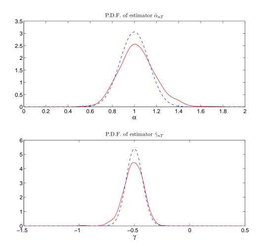
The solid lines give the pdf of the semiparametrically efficient estimators of parameter  $\gamma$  (upper Panel, true value 1) and parameter  $\alpha$  (lower Panel, true value -0.5). The pdf is computed by a kernel density estimator. Sample sizes are n=200 and T=20. The dashed lines in the two Panels give the pdf of a normal distribution centered at the true value of the parameter and with variance equal to the semi-parametric efficiency bound divided by nT.
